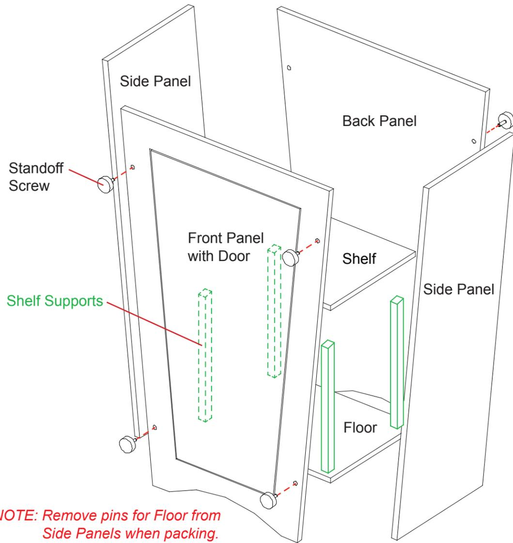
*NOTE: Remove pins for Floor from Side Panels when packing.*
