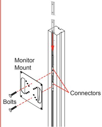
Slide Connectors into groove of Extrusion. Tighten Set Screws to secure in place. Attach Monitor Mount back plate to Extrusion, using bolts.
