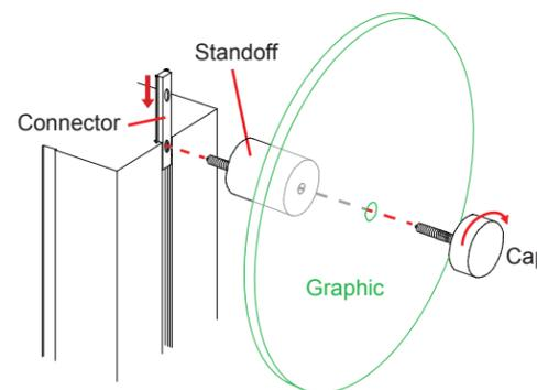
Slide Connector into groove of Vertical Extrusion. Tighten set screws to secure in place. Screw Standoff into Connector. Place Graphic between Standoff and Cap then screw Cap to tighten in place.
