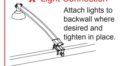
Attach lights to backwall where desired and tighten in place.
